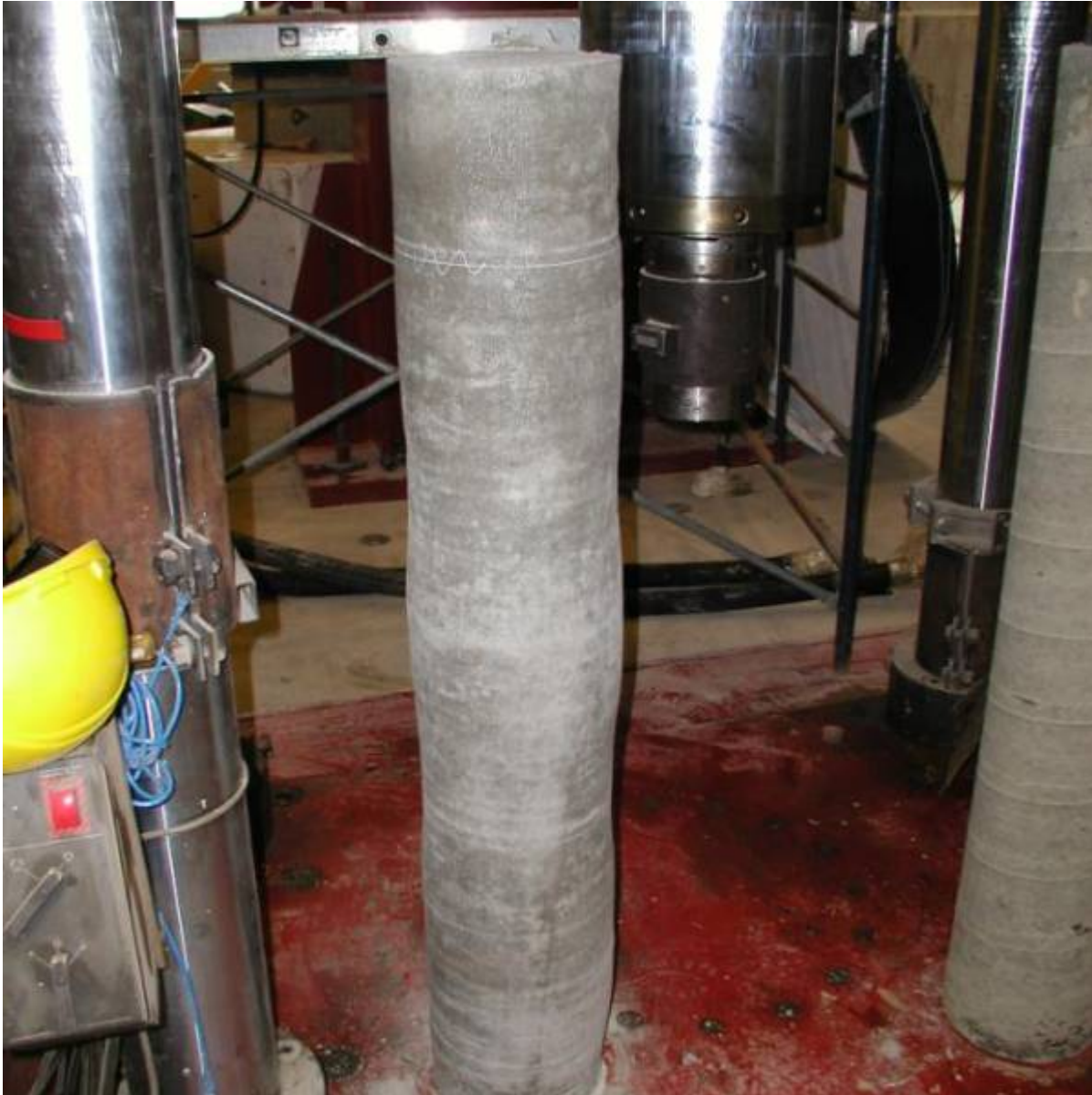
Figure 67: Bulged concrete column.
