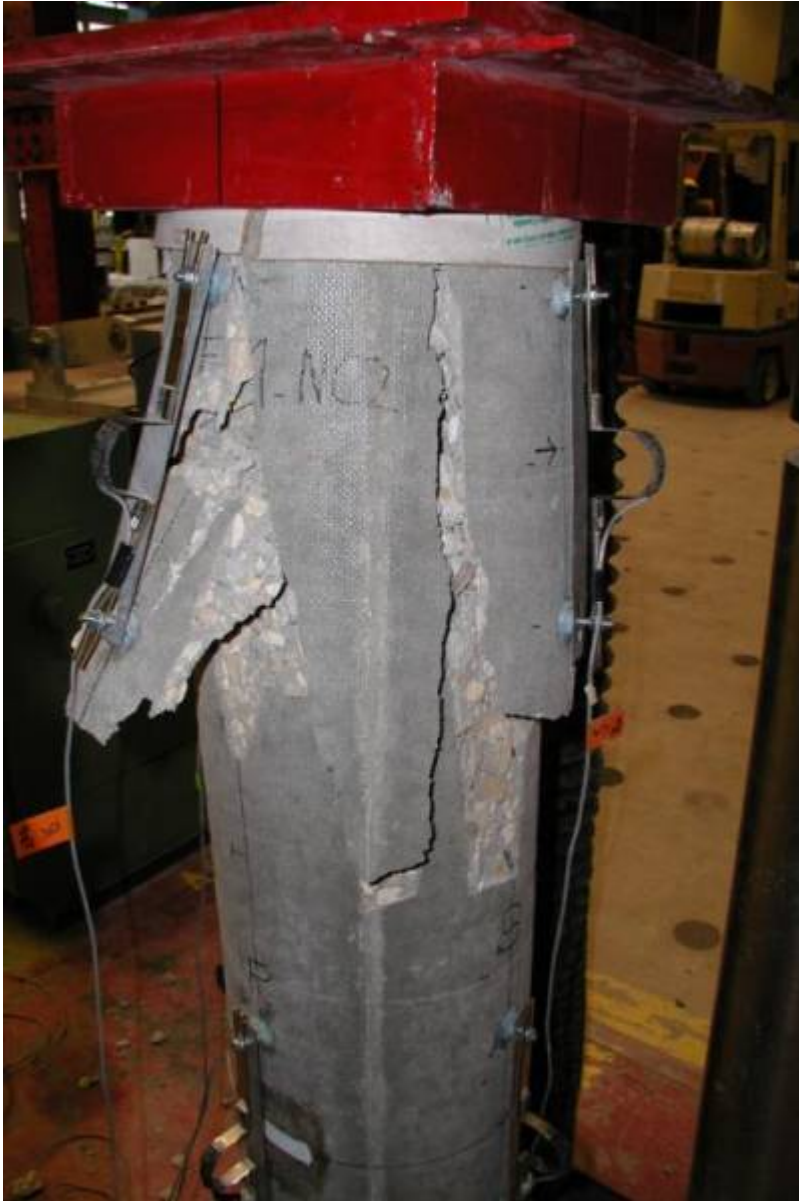
Figure 64: Column FF-NC-2 after failure.
