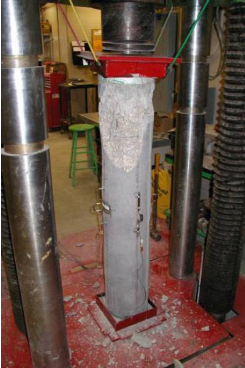
Figure 65: Column FF-NC-1 after failure.
