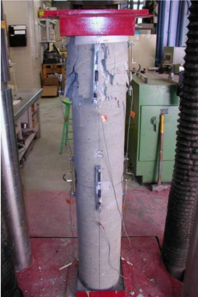
Figure 65: Column CT-NC-2 after failure.
